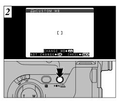
Using the light source for which you want to set the white balance, hold a sheet of white paper so that it fills the entire screen.
